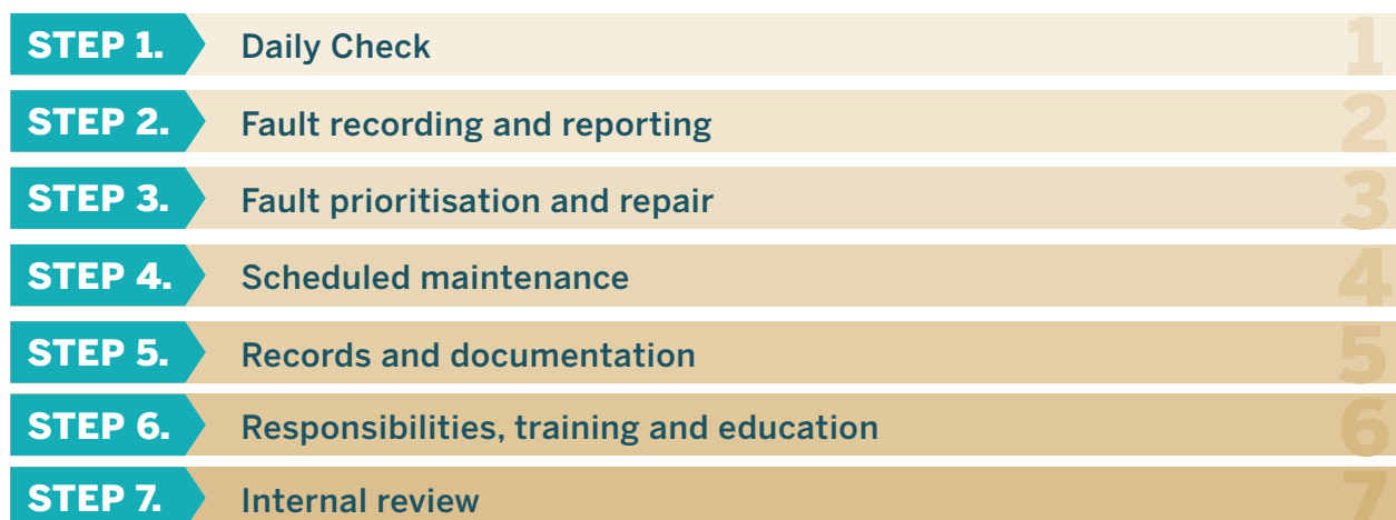
Figure 7 Maintenance management system
