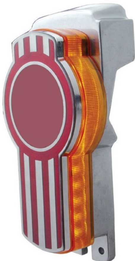
Figure 1: Example of backlit badge fitted with a yellow light
