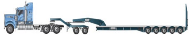
Figure 3: Example of a prime mover, low loader dolly, and 5-axle low loader
